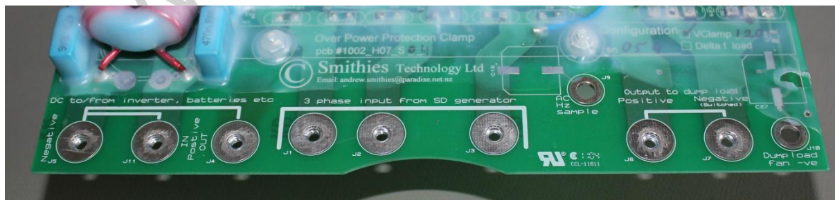
Close up view of revised version of ME or GE circuit board with integrated output diode.
