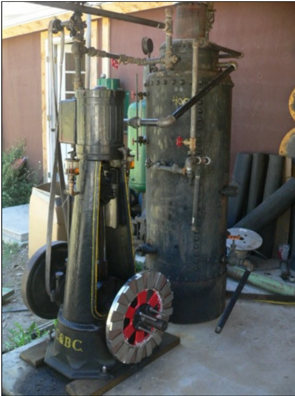
There is the back magnet rotor mounted to the shaft of the engine.
