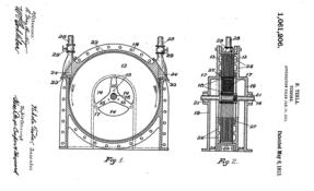
Figure 1.: American Patent No. 1,061,206 of Tesla turbine [1].
