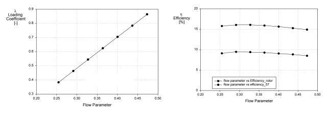
Figure 16.: Loading coefficient for turbulent solution, turbine.
